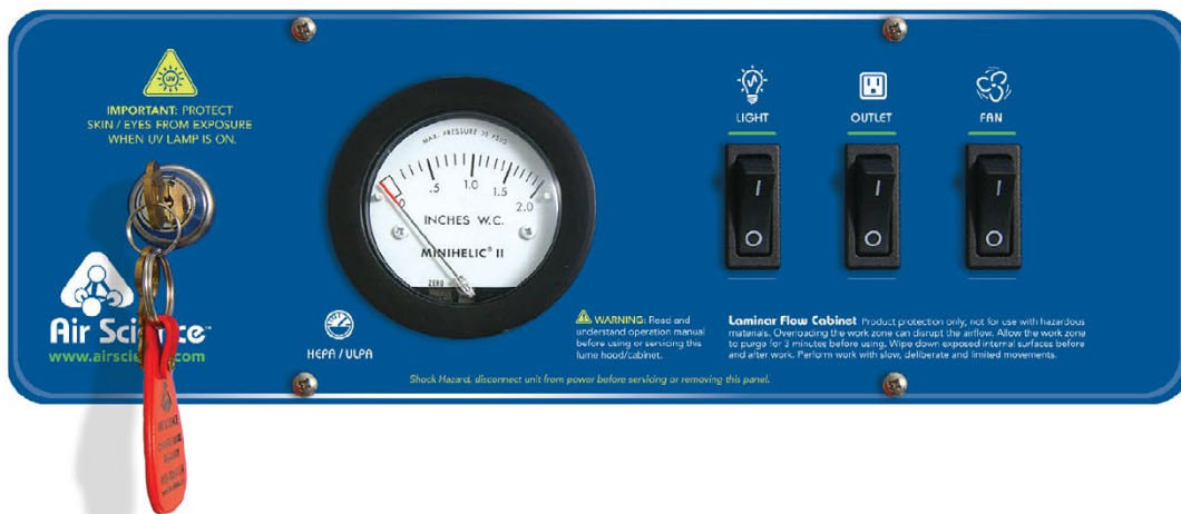
Control panel On/Off switch for fan, lighting, GFCI outlets, Minihelic UHPA pressure gauge to measure filter performance, UV lamp key switch.
